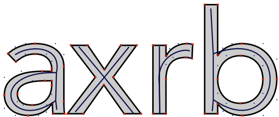
Figure 2. Skeletons of several letters. Curves and nodes can be shared by different strokes.
